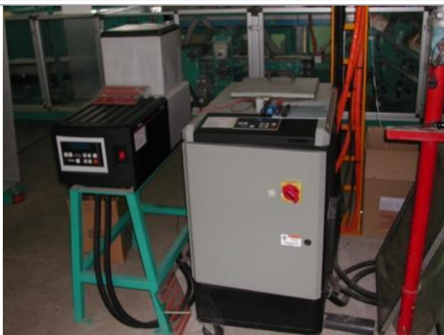
Hot-melt glue system
